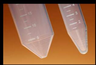
Engraved graduation on the cone, allowing easy reading of small volumes
