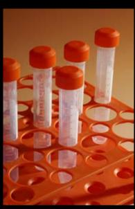
Special rack holding either 20 x 50 ml tubes or 30 x 15 ml tubes, or a mix
